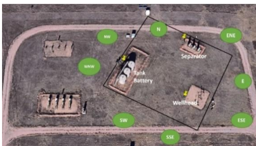
Figure 1 METEC R3 Test Pad
