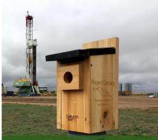
A Project Canary emissionsmonitoring device shown near an oil and gas drilling rig.
